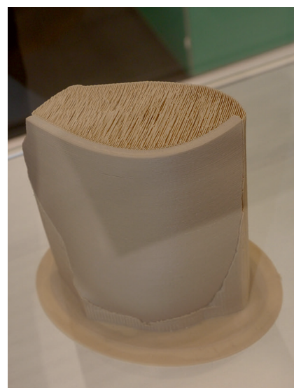
Fig. 2. Skull implants of PEEK. The support structures behind it are so loosely designed, they can be mechanically detached.
