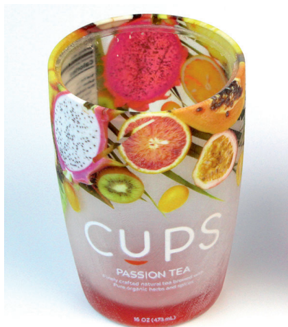
Fig. 1. PolyJet printing allows designers to create full-color packaging with integrated graphics and labels in one step. © Strataysys
